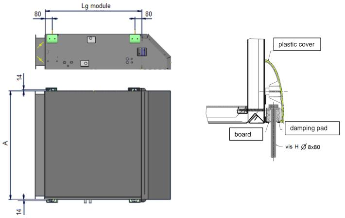
Assembling the casings (for multi-unit AHUs):
