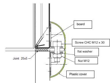
Assembly between caissons and plate recuperator block HEE :
