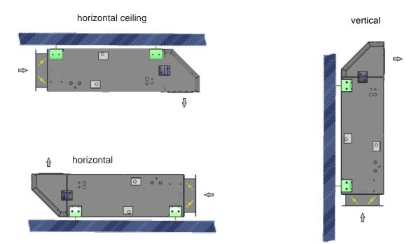
Depending on the type of unit being controlled, it can either be ceiling- or floor-mounted or installed vertically.
